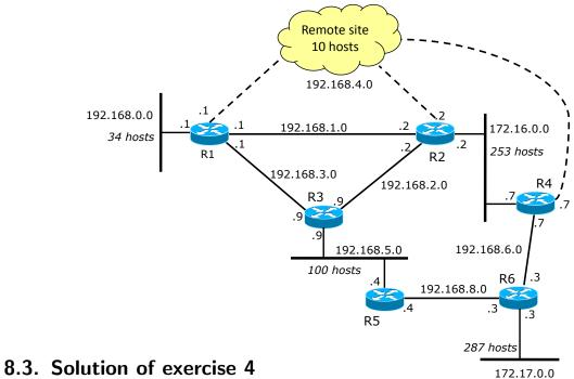
The topology includes only class C networks, excluding the LIN with 300 elements that has to be handled with a class B block. The solution is shown in the figure below.
