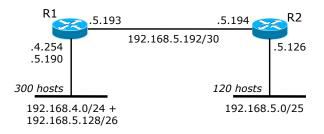
It is worthy noting that, even if it would be possible to partition the original LINs into even smaller portions (for example the network with 300 hosts could be partitioned into 253 + 29 + 13 + 5, i.e., a /26 + /27 + /28 + /29 network), this is not a good idea as it adds more complexity while a coarse partitioning was enough to make everthing working.
