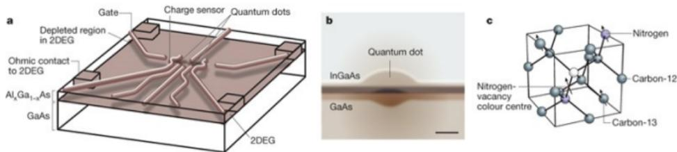
Quantum dot and solid-state dopant qubits. (a) An electrostatically confined quantum dot; the structure shown is several  $\mu\text{m}$  across. 2DEG, two-dimensional electron gas. (b) A self-assembled quantum dot. Scale bar,  $\sim 5\text{nm}$ . (c) The atomic structure of a nitrogen-vacancy centre in the diamond lattice, with lattice constant 3.6 Å.
