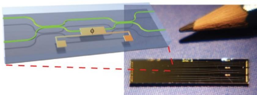
A microchip containing several silica-based waveguide interferometers with thermo-optic controlled phase shifts for photonic quantum gates. Green lines show optical waveguides; yellow components are metallic contacts. Pencil tip shown for scale.
