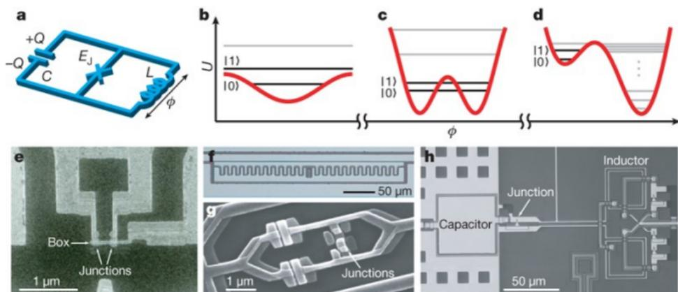
In superconductors at low temperature, electrons bind into Cooper pairs that condense into a state with zero-resistance current and a well-defined phase. In superconducting circuits, the potential for the quantum variables of that Cooper-pair condensate may be changed by controlling macroscopically defined inductances ( $L$ ), capacitances ( $C$ ) and so on, allowing the construction of qubits.
