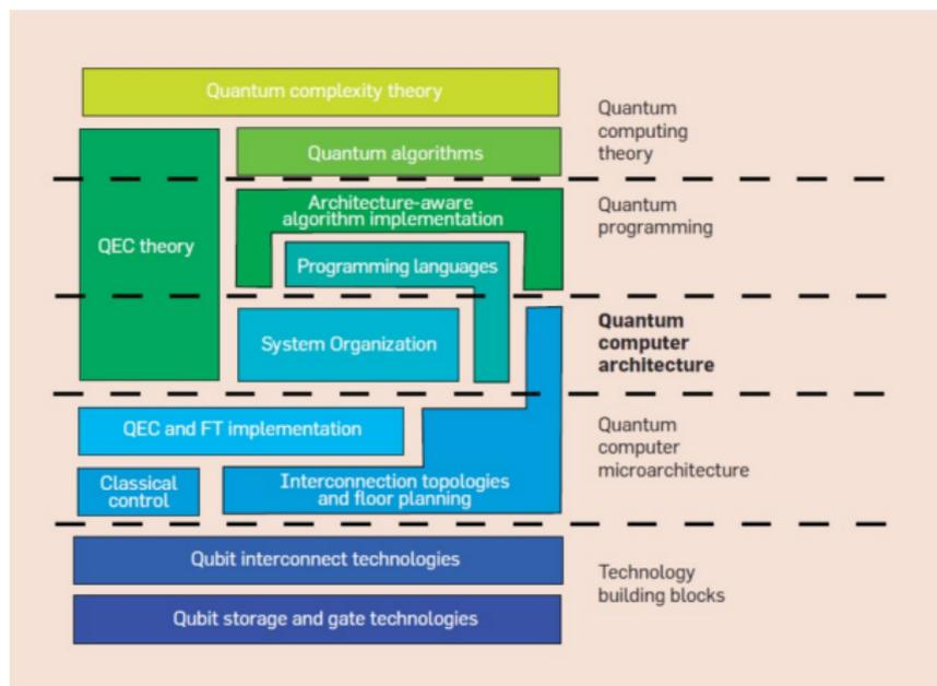
At the bottom of the stack we have the technologies for storing, processing or transporting individual qubits.
